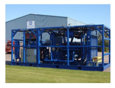
AXON Well Intervention Products' HD-500 precision balanced multi-purpose triplex plunger pump is a proven solution for a wide range of applications, including fracturing, cementing, acidizing, pumping, coil tubing, and IWOC systems.
