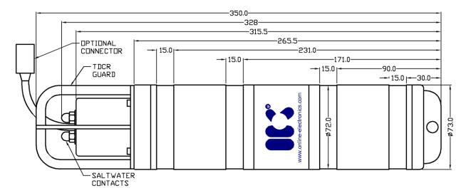
The standard 800 Series model is can produce up to 20W of acoustic power and has a single operating frequency in the range of 24-30 kHz (configured at time of manufacture). In addition to the standard model, a number of alternative configurations are available that offer additional functionality and/or performance:
